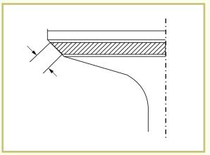
If the contact area appears to be closer to the bottom of the valve seat, you should narrow the seat from the top, thus helping to center the contact area. Likewise, if the contact area is closer to the top of the valve seat, you can center the contact area by narrowing the seat from the bottom. Examples of this are shown in Figure 28.
