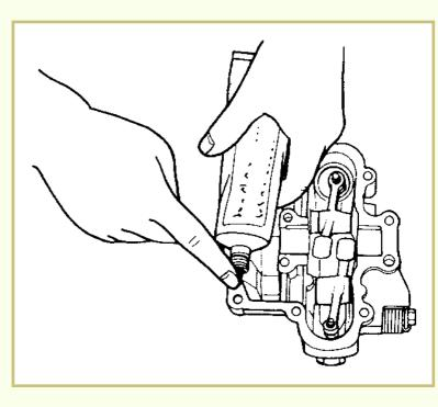
**2** Once sealed, install the cover and tighten the mounting bolts in the sequence shown.
