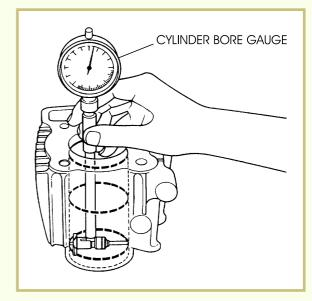
Insert the cylinder bore gauge at a point near the top of the cylinder and take a reading of the micrometer. The gauge is then moved to a point near the center of the cylinder and a reading is taken there as well. Finally, the gauge is positioned at the bottom of the cylinder and another reading is taken. This is done for both the X and Y axis measurements to determine the cylinder's trueness (Figure 10). The readings are compared and the difference indicates the amount of wear.
