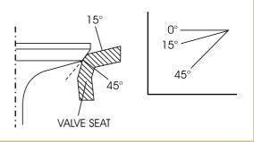
The most common hand tools used to refinish a valve seat are pictured in Figure 23. The appropriate angle for a valve seat is found in the service manual for the motorcycle or ATV engine. The equipment for valve seat grinding is normally available from specialty tool manufacturers or from automotive supply stores.
