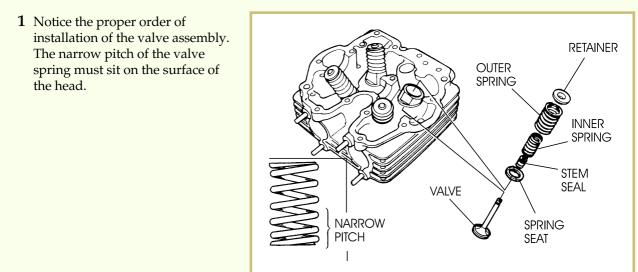
**2** Reassemble the valves, using a valve spring compressor to hold the springs while installing valve keepers.
