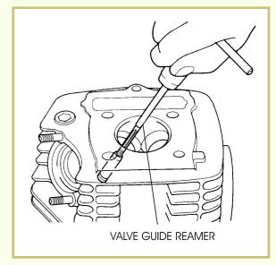
The appropriate inside diameter of a valve guide depends on the size of the valve stem. The service manual for the engine specifies the proper diameter. This allows sufficient clearance for the stem to move through the guide as the valve opens and closes. After a valve guide has been reamed, any metal particles should be removed with compressed air. Then the area should be washed with solvent.
