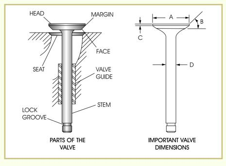
Valves must operate under a variety of extreme conditions. As a result, certain areas of the valve assembly often show signs of wear or physical damage. Because they're located in the combustion chamber, valves can reach temperatures of well over 1,000 degrees Fahrenheit under normal operating conditions! It's not surprising that they can actually begin to melt under these high temperatures. Heat tends to wear away the exposed surfaces, particularly the valve heads.
