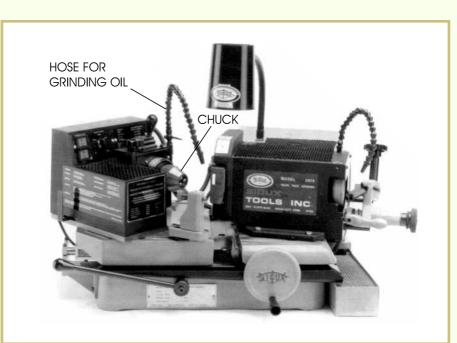
FIGURE 17—A Typical Valve Grinding Machine (Courtesy of Sioux Tools, Inc.)
