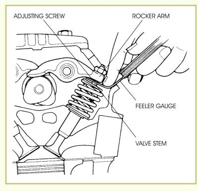
2 Adjust the clearance using the adjusting screw and locknut. The actual adjustment procedure for four-stroke motorcycle and ATV valves is discussed in detail in a later study unit.
