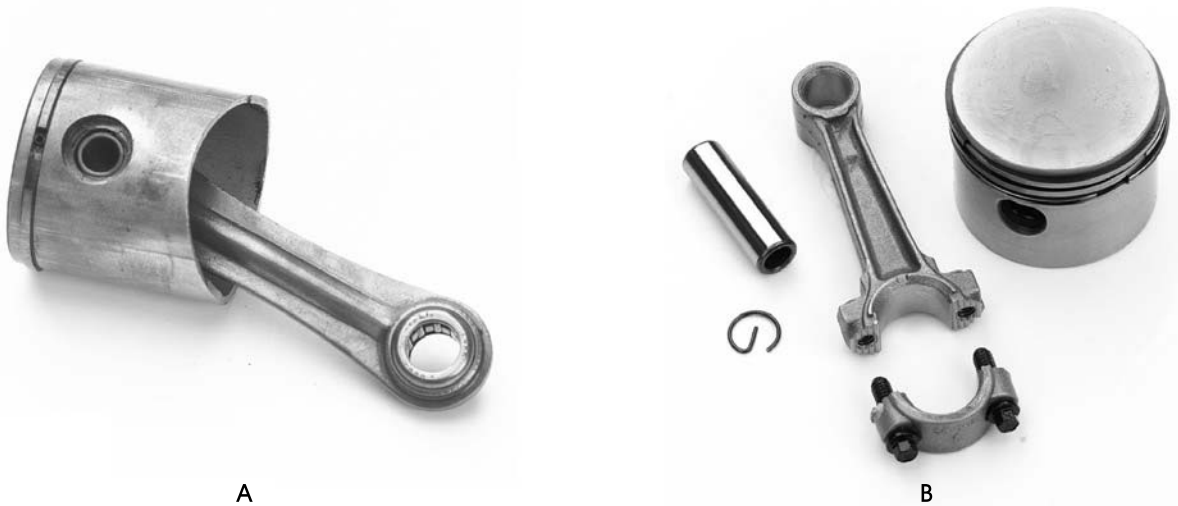
FIGURE 24 —This illustration shows the two types of connecting rods. Figure 24A shows a one-piece connecting rod with the piston attached. Figure 24B shows a multi-piece connecting rod with the piston detached.
