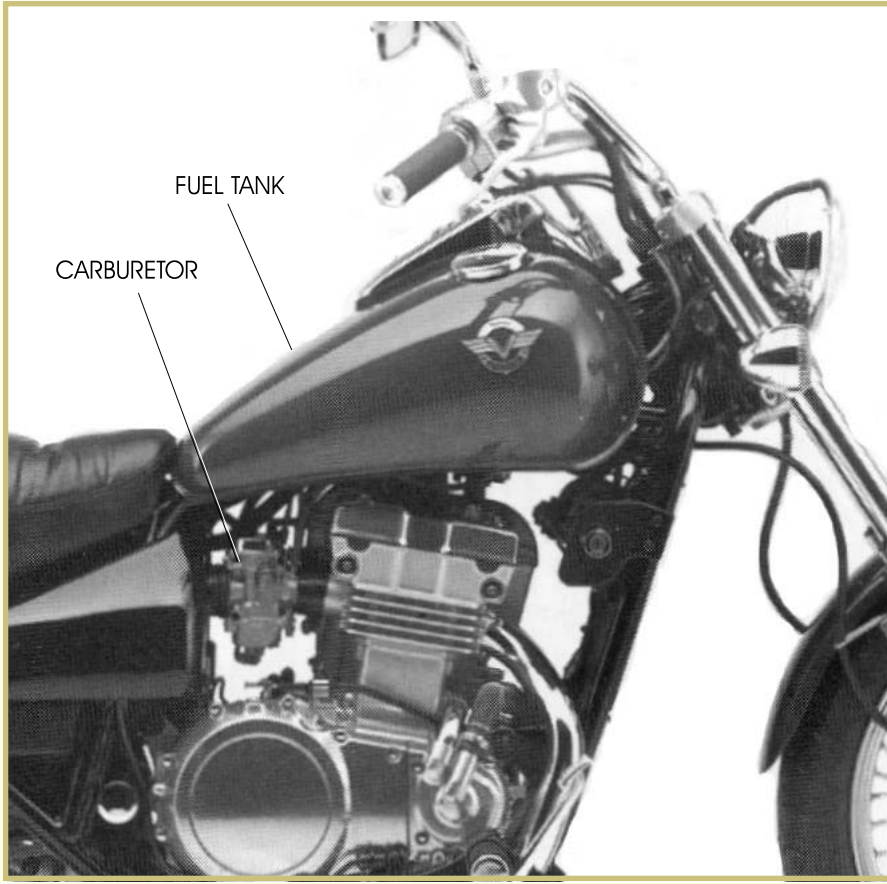
FIGURE 5—The fuel tank is used to store gasoline, and is mounted above the engine and carburetor in this photograph. (Courtesy Kawasaki Motor Corp., U.S.A.)
