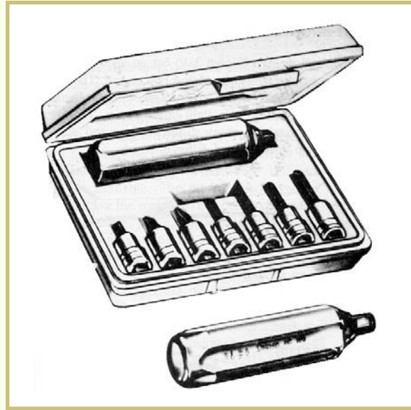
FIGURE 26 —This illustration shows a typical impact screwdriver.
