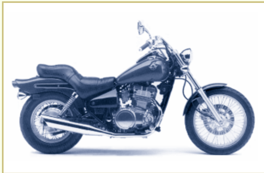
FIGURE 2—A medium (500 cc) custom cruiser. Note the laid-back riding position. (Courtesy of Kawasaki Motor Corp., U.S.A.)
