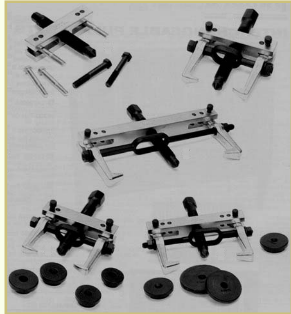
FIGURE 43—Pullers come in various shapes and sizes. (Courtesy of Snap-On Tool Company, copyright owner.)
