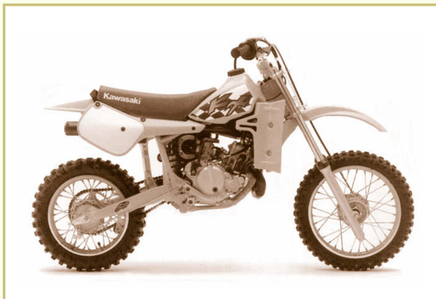
FIGURE 9—Off-road motorcycles come in various shapes and sizes. This is a small 50 cc off-road motorcycle. (Courtesy of Kawasaki Motor Corp., U.S.A.)
