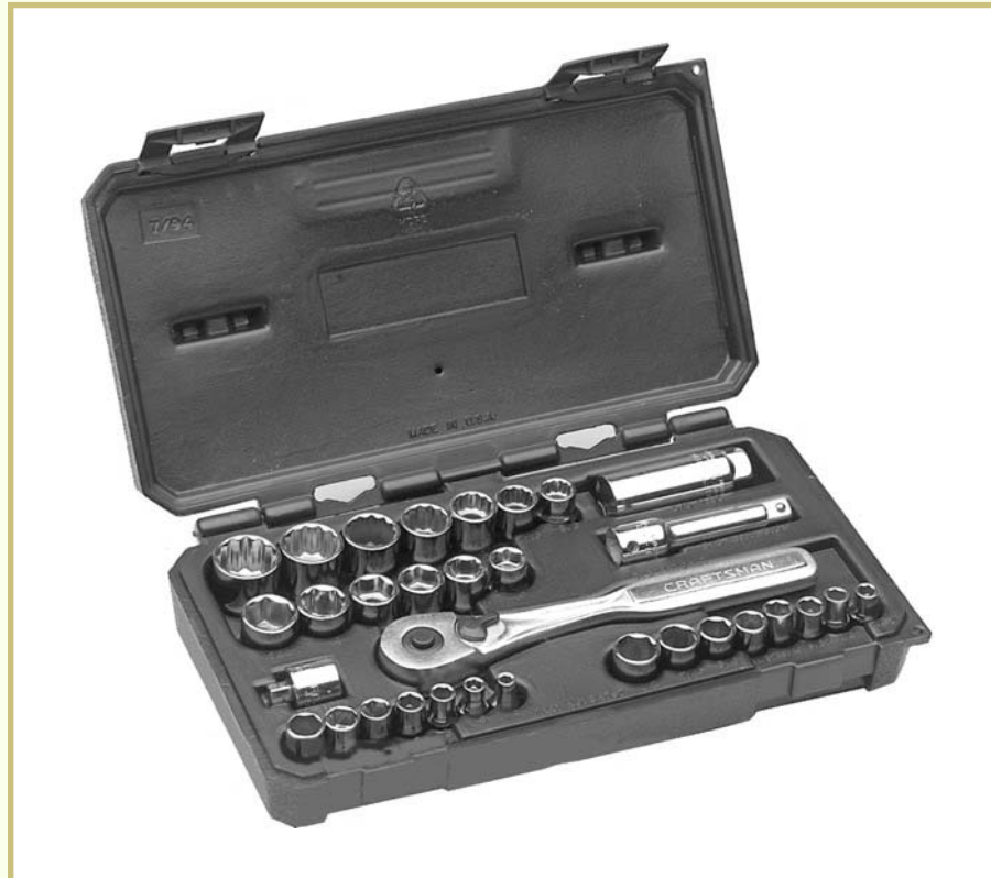
FIGURE 17—This is a typical set of socket wrenches. (Courtesy of Sears Craftsman)
