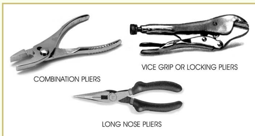
FIGURE 27 —This illustration shows combination slip-joint pliers (A); locking pliers (B); and long nose pliers (C).
