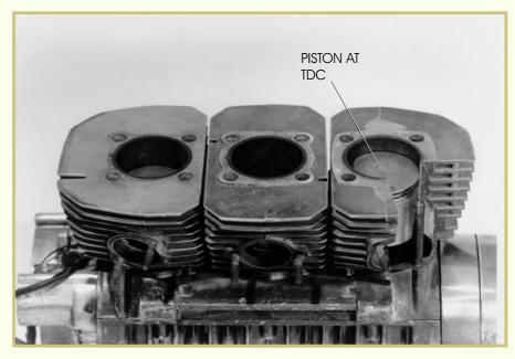
FIGURE 23—A 120° crankshaft has one piston at TDC every 120 degrees. This provides three power strokes in one crankshaft revolution.
