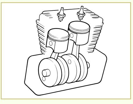
FIGURE 21—A 180-degree crankshaft design has one piston at TDC while the other piston is at BDC as illustrated here.
