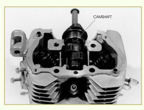
FIGURE 34—This picture shows a double overhead camshaft.
