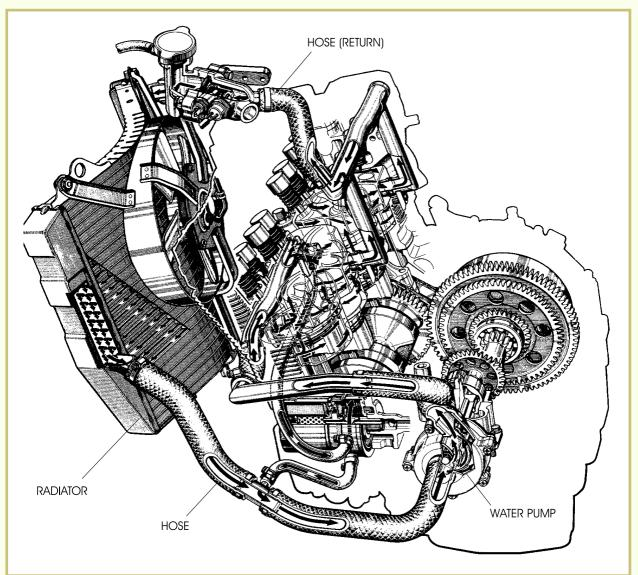
FIGURE 37—This illustration shows the system components in a four-stroke liquid-cooled engine.
