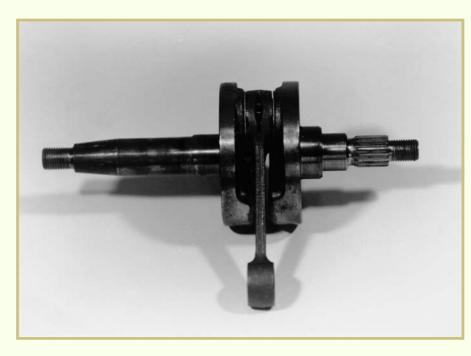
FIGURE 27—This illustration shows a one-piece four-stroke crankshaft.
