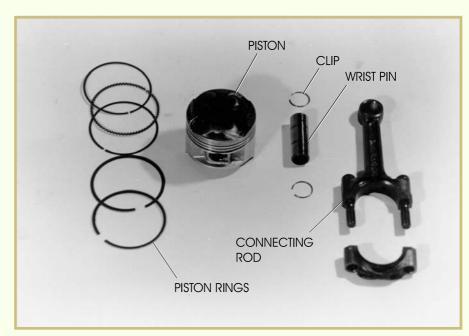
FIGURE 30—This picture shows a four-stroke piston and its related parts.
