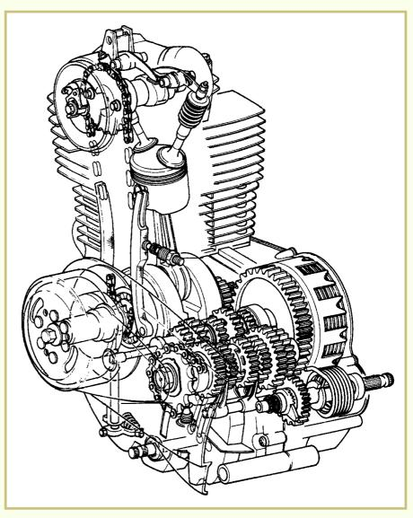
The bottom end of a four-stroke engine contains the heart of the engine the crankshaft. The four-stroke crankshaft may be made up of two flywheel halves (Figure 26), or it may be a one-piece design (Figure 27). It will have a connecting rod, rod (*crank*) pin (if it's a multi-piece design), and a connecting rod needle bearing. At least one bearing on each end supports the crankshaft and allows it to rotate freely. The crankshaft is located in the engine crankcases.
