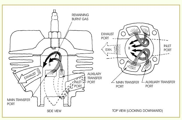
FIGURE 14—The ports in a two-stroke cylinder allow the flow of gases in and out of the engine.
