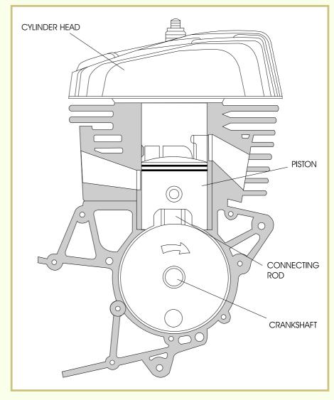
The bottom end of a two-stroke engine contains the heart of the engine the crankshaft. The two-stroke *crankshaft* is made up of two flywheel halves, a connecting rod, a connecting rod pin, and a connecting rod bearing (Figure 8). A bearing on each end supports the crankshaft and allows it to rotate. The crankshaft is located inside the engine crankcases.
