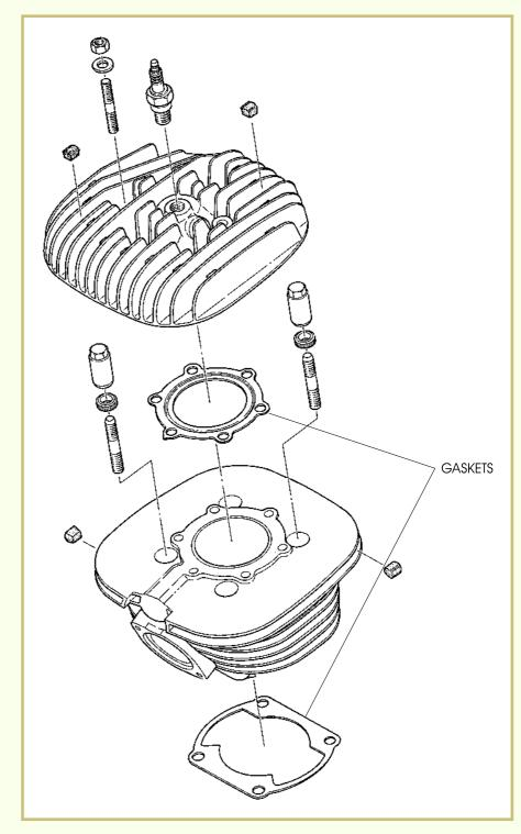
FIGURE 12—This illustration shows typical gaskets found on engine mating surfaces. The last part of the bottom end is the *starting mechanism*. The twostroke engine uses one of three different starting mechanisms. A *kick starter* has an external lever on the side crankcase. The rider pushes the lever down with his or her foot to turn the crankshaft. Turning the crankshaft starts the engine.
