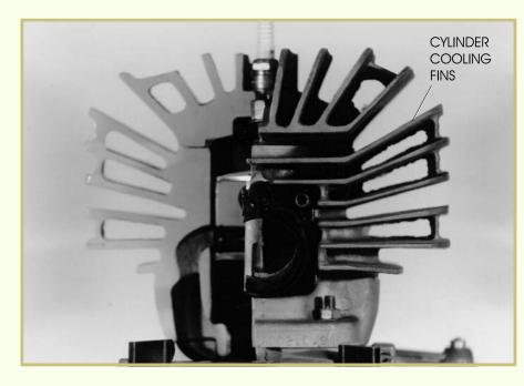
FIGURE 16—A forced draft air-cooled engine uses an engine-driven fan to move air.
