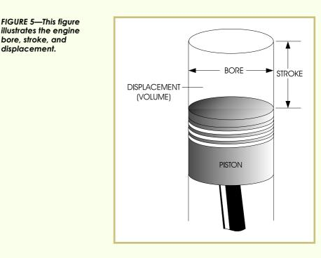
You can calculate the displacement of an engine if you know the diameter of the cylinder and the length of the stroke of the engine. The displacement of an engine can be calculated by using the following formula:
