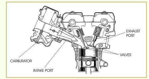
FIGURE 32—The four-stroke cylinder head has ports and valves to allow the flow of intake and exhaust gases. FIGURE 33—This picture shows a single overhead camshaft.
