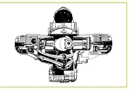
FIGURE 39—A horizontallyopposed twin is illustrated here. Note the 180° crankshaft design.
