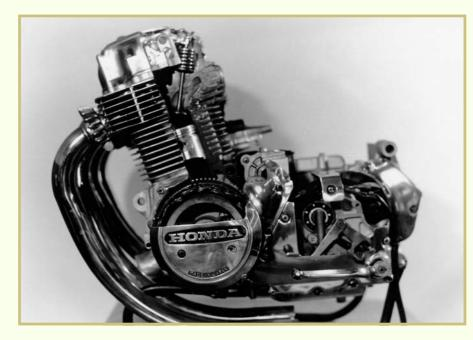
FIGURE 36—Cylinder and cylinder head cooling fins control temperatures on the air-cooled engine. (Copyright by American Honda Motor Co., Inc. and reprinted with permission)
