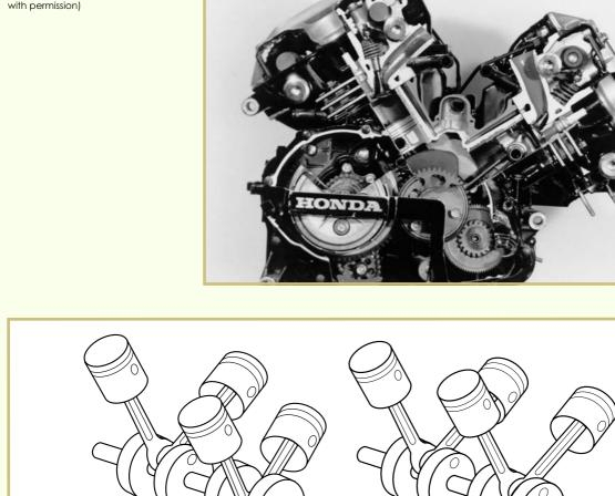
FIGURE 42—This illustration shows the V-four, four-stroke, 180° and 360° crankshaft designs.
