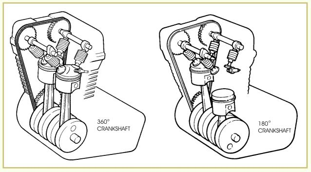
FIGURE 38—A four-stroke, twin-cylinder, 180° crankshaft design is shown on the right. A 360° design is shown on the left.
