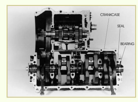
Seals are used to protect rotating shaft bearings. The seals are typically located at the ends of the rotating shafts. These seals prevent gases and oil from escaping from the crankcases and also prevent outside substances from getting into the crankcases.
