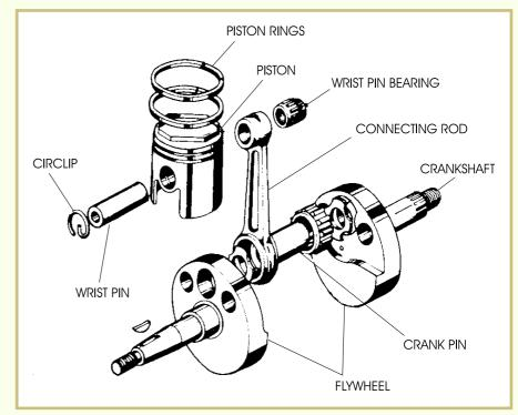
FIGURE 13—The piston and its related parts are attached to the crankshaft connecting rod.
