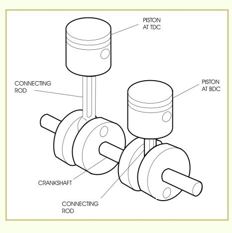
FIGURE 22—Although not very common, some twostrokes are produced in a V-twin configuration.
