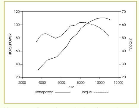
More torque usually means better acceleration and more towing capacity. Higher horsepower usually means a higher top speed. The amount of horsepower and torque an engine develops depends on many design factors. The displacement, compression ratio, fuel mixture, engine design, ignition timing, and valve timing (on four-stroke engines) all affect horsepower and torque.
