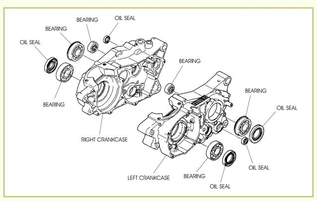
FIGURE 10—This illustration shows the seals and bearings located in the crankcases.
