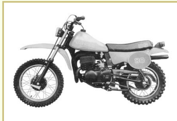
FIGURE 2—The Suzuki DS 80 motorcycle is being used for our air-cooled two-stroke engine
